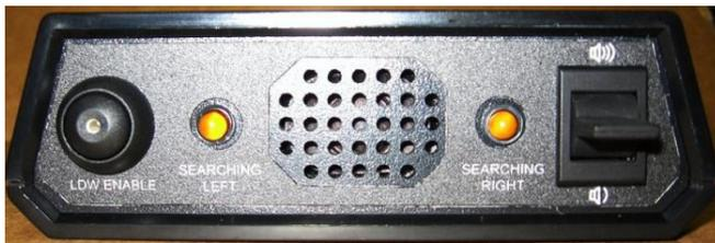
The SafeTraK 3 Truck Interface Module consists of a LDW Enable push button with GREEN indicator, two AMBER searching indicators, a volume switch and a speaker. For optimal performance the Truck Interface Module should not be covered or blocked in any fashion.
