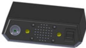
The SafeTraK 3 Truck Interface Module (TIM) is intended to support the Takata SafeTraK 3 Lane Departure Warning System. The TIM provides the switches, indicators and speaker for trucks which do not have these features factory installed.
